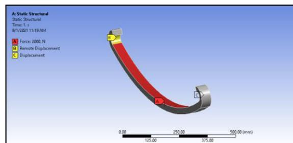
Figure 4: Boundary conditions applied on leaf spring
