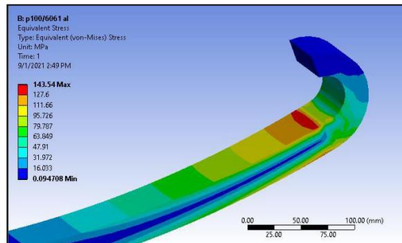
Figure 7: Equivalent stress plot of mono leaf spring using aluminium composite material
