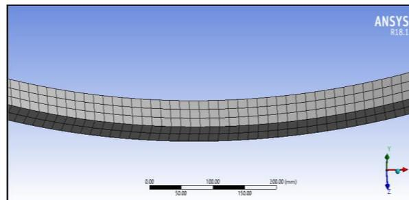
Figure 3: Meshed model of leaf spring
