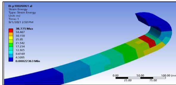
Figure 8: Strain energy plot of mono leaf spring using aluminium composite material
