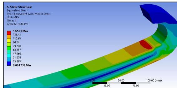
Figure 5: Equivalent stress plot for steel
