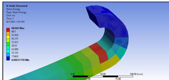
Figure 6: Strain energy plot of mono leaf spring
